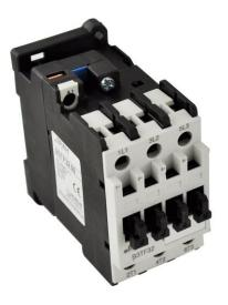
PART NUMBER – B3TF3211: BRAH Electric, aftermarket direct replacement contactors for Siemens 3TF3211, World Series, type 3TF, 3P, 3PH, 16A, 600V, 5HP @ 230V, 10HP @ 460V, 15HP @ 575V, complete with 110/120V AC coil, 1 N/O - 1 N/C auxiliary contact, AC magnetic contactor, suitable for use with 3TF series motor control systems
