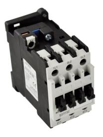
PART NUMBER – B3TF3211-0AK6: BRAH Electric, aftermarket direct replacement contactors for Siemens 3TF3211-0AK6, World Series, type 3TF, 3P, 3PH, 16A, 600V, 5HP @ 230V, 10HP @ 460V, 15HP @ 575V, complete with 110/120V AC coil, 1 N/O - 1 N/C auxiliary contact, AC magnetic contactor, suitable for use with 3TF series motor control systems
