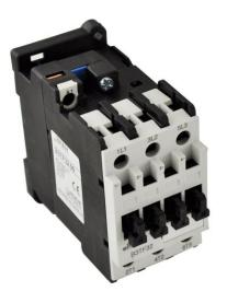
PART NUMBER – B3TF3211-0AP6: BRAH Electric, aftermarket direct replacement contactors for Siemens 3TF3211-0AP6, World Series, type 3TF, 3P, 3PH, 16A, 600V, 5HP @ 230V, 10HP @ 460V, 15HP @ 575V, complete with 240V AC coil, 1 N/O - 1 N/C auxiliary contact, AC magnetic contactor, suitable for use with 3TF series motor control systems
