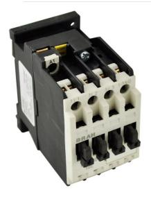
PART NUMBER – B3TF33: BRAH Electric, aftermarket direct replacement contactors for Siemens 3TF33, World Series type 3TF, 3P, 3PH, 22A, 600V, 7.5HP @ 230V,15HP @ 460V, 20HP @ 575V, complete with 110/120V AC Coil, 1 N/O -1N/C auxiliary contact, AC magnetic contactor, suitable for use with 3TF series motor control systems
