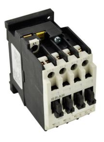
PART NUMBER – B3TF3311-0AK6: BRAH Electric, aftermarket direct replacement contactors for Siemens 3TF3311-0AK6, World Series type 3TF, 3P, 3PH, 22A, 600V, 7.5HP @ 230V,15HP @ 460V, 20HP @ 575V, complete with 110/120V AC Coil, 1 N/O -1N/C auxiliary contact, AC magnetic contactor, suitable for use with 3TF series motor control systems
