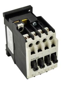
PART NUMBER – B3TF3311-0AP6: BRAH Electric, aftermarket direct replacement contactors for Siemens 3TF3311-0AP6, World Series type 3TF, 3P, 3PH, 22A, 600V, 7.5HP @ 230V,15HP @ 460V, 20HP @ 575V, complete with 240V AC Coil, 1 N/O -1N/C auxiliary contact, AC magnetic contactor, suitable for use with 3TF series motor control systems
