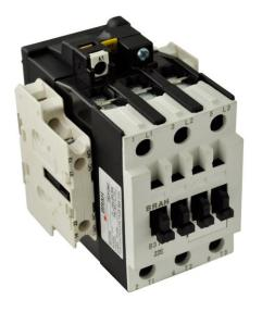
PART NUMBER – B3TF3422: BRAH Electric, aftermarket direct replacement contactors for Siemens 3TF3422, World Series type 3TF, 3P, 3PH, 32A, 600V, 10HP @ 230V,20HP @ 460V, 30HP @ 575V, complete with 110/120V AC Coil, 2 N/O – 2N/C auxiliary contact, AC magnetic contactor, suitable for use with 3TF series motor control systems
