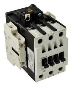
**PART NUMBER – B3TF3422-OAC2**: BRAH Electric, aftermarket direct replacement contactors for Siemens 3TF3422-OAC2, World Series type 3TF, 3P, 3PH, 32A, 600V, 10HP @ 230V,20HP @ 460V, 30HP @ 575V, complete with 24V AC Coil, 2 N/O – 2N/C auxiliary contact, AC magnetic contactor, suitable for use with 3TF series motor control systems
