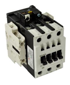
PART NUMBER – B3TF3422-0AK6: BRAH Electric, aftermarket direct replacement contactors for Siemens 3TF3422-0AK6, World Series type 3TF, 3P, 3PH, 32A, 600V, 10HP @ 230V,20HP @ 460V, 30HP @ 575V, complete with 110/120V AC Coil, 2 N/O – 2N/C auxiliary contact, AC magnetic contactor, suitable for use with 3TF series motor control systems
