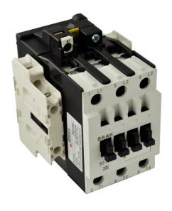
PART NUMBER – B3TF3422-0AP6: BRAH Electric, aftermarket direct replacement contactors for Siemens 3TF3422-0AP6, World Series type 3TF, 3P, 3PH, 32A, 600V, 10HP @ 230V,20HP @ 460V, 30HP @ 575V, complete with 240V AC Coil, 2 N/O – 2N/C auxiliary contact, AC magnetic contactor, suitable for use with 3TF series motor control systems
