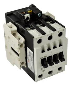
PART NUMBER – B3TF3522-OAC2: BRAH Electric, aftermarket direct replacement contactors for Siemens 3TF3522-OAC2, World Series type 3TF, 3P, 3PH, 38A, 600V, 15HP @ 230V,25HP @ 460V, 30HP @ 575V, complete with 24V AC Coil, 2 N/O-2 N/C auxiliary contact, AC magnetic contactor, suitable for use with 3TF series motor control systems
