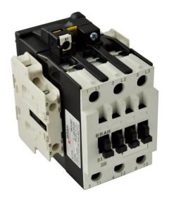
PART NUMBER – B3TF3522-0AP6: BRAH Electric, aftermarket direct replacement contactors for Siemens 3TF3522-0AP6, World Series type 3TF, 3P, 3PH, 38A, 600V, 15HP @ 230V,25HP @ 460V, 30HP @ 575V, complete with 240V AC Coil, 2 N/O-2 N/C auxiliary contact, AC magnetic contactor, suitable for use with 3TF series motor control systems
