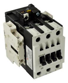
PART NUMBER – B3TF3522-0AVO: BRAH Electric, aftermarket direct replacement contactors for Siemens 3TF3522-0AVO, World Series type 3TF, 3P, 3PH, 38A, 600V, 15HP @ 230V,25HP @ 460V, 30HP @ 575V, complete with 480V AC Coil, 2 N/O-2 N/C auxiliary contact, AC magnetic contactor, suitable for use with 3TF series motor control systems
