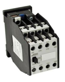
PART NUMBER – B3TF41: BRAH Electric, aftermarket direct replacement contactors for Siemens 3TF41, World Series, type 3TF, 3P, 3PH, 12A, 600V, 3HP @ 230V, 7.5HP @ 460V, 10HP @ 575V, complete with 110/120V AC coil, 2 N/O - 2 N/C auxiliary contact, AC magnetic contactor, suitable for use with 3TF series motor control systems
