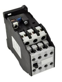
PART NUMBER – B3TF4122: BRAH Electric, aftermarket direct replacement contactors for Siemens 3TF4122, World Series type 3TF, 3P, 3PH, 12A, 600V, 3HP @ 230V,7.5HP @ 460V, 10HP @ 575V, complete with 110/120V AC Coil,2 N/O - 2 N/C auxiliary contact, AC magnetic contactor, suitable for use with 3TF series motor control systems
