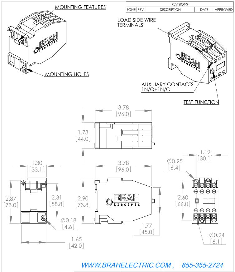
\*NOTE: BRAH ELECTRIC CONTACTOR B3TF4122-0AV0 IS AN AFTERMARKET DIRECT REPLACMENT FOR SIEMENS 3TF4122-0AV0,3TF SERIES. SUITABLE FOR USE WITH 3TF SERIES MOTOR CONTROL SYSTEMS
