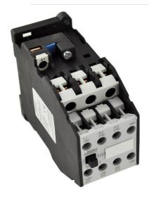
PART NUMBER – B3TF4122-0AVO: BRAH Electric, aftermarket direct replacement contactors for Siemens 3TF4122-0AVO, World Series, type 3TF, 3P, 3PH, 12A, 600V, 3HP @ 230V, 7.5HP @ 460V, 10HP @ 575V, complete with 480V AC coil, 2 N/O - 2 N/C auxiliary contact, AC magnetic contactor, suitable for use with 3TF series motor control systems
