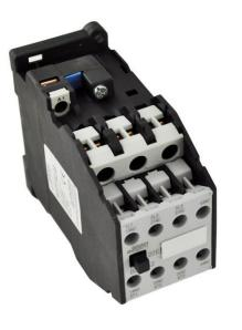
PART NUMBER – B3TF42: BRAH Electric, aftermarket direct replacement contactors for Siemens 3TF42, World Series, type 3TF, 3P, 3PH, 16A, 600V, 5HP @ 230V, 10HP @ 460V, 15HP @ 575V, complete with 110/120V AC coil, 2 N/O - 2 N/C auxiliary contact, AC magnetic contactor, suitable for use with 3TF series motor control systems
