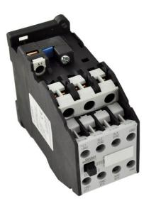
PART NUMBER – B3TF4222: BRAH Electric, aftermarket direct replacement contactors for Siemens 3TF42, World Series, type 3TF, 3P, 3PH, 16A, 600V, 5HP @ 230V, 10HP @ 460V, 15HP @ 575V, complete with 110/120V AC coil, 2 N/O - 2 N/C auxiliary contact, AC magnetic contactor, suitable for use with 3TF series motor control systems
