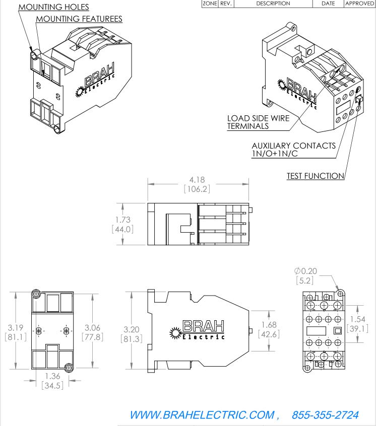
\*NOTE: BRAH ELECTRIC CONTACTOR B3TF4222-0AC2 IS AN AFTERMARKET DIRECT REPLACMENT FOR SIEMENS 3TF4222-0AC2,3TF SERIES. SUITABLE FOR USE WITH 3TF SERIES MOTOR CONTROL
