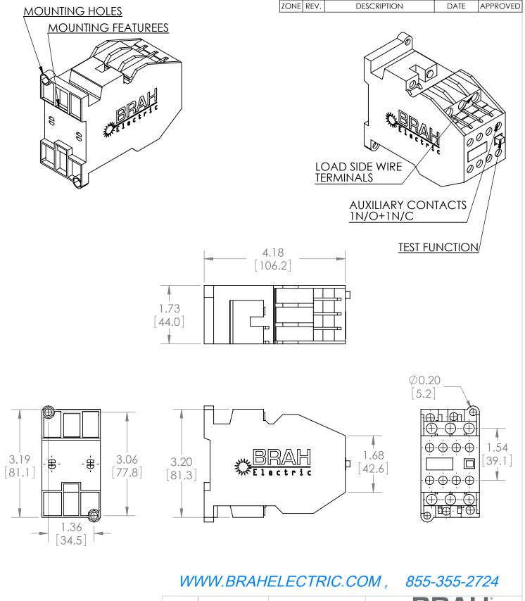
\*NOTE: BRAH ELECTRIC CONTACTOR B3TF4222-0AK6 IS AN AFTERMARKET DIRECT REPLACMENT FOR SIEMENS 3TF4222-0AK6,3TF SERIES. SUITABLE FOR USE WITH 3TF SERIES MOTOR CONTROL SYSTEMS
