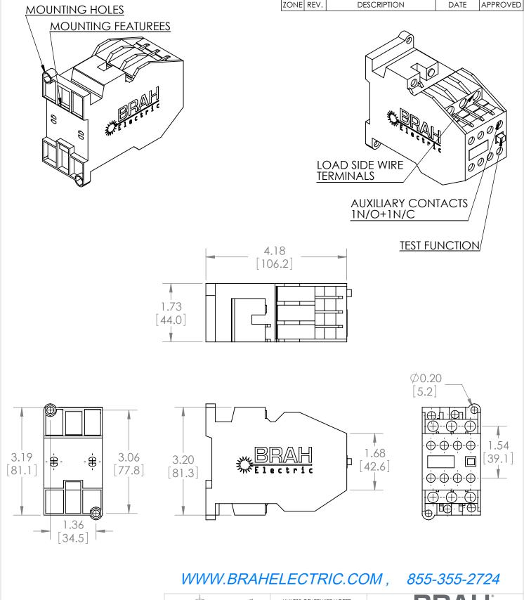
\*NOTE: BRAH ELECTRIC CONTACTOR B3TF4222-0AV0 IS AN AFTERMARKET DIRECT REPLACMENT FOR SIEMENS 3TF4222-0AV0,3TF SERIES. SUITABLE FOR USE WITH 3TF SERIES MOTOR CONTROL **SYSTEMS**
