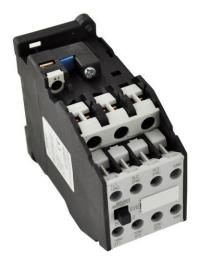
PART NUMBER – B3TF4322: BRAH Electric, aftermarket direct replacement contactors for Siemens 3TF4322, World Series, type 3TF, 3P, 3PH, 22A, 600V, 7.5HP @ 230V, 15HP @ 460V, 20HP @ 575V, complete with 110/120V AC coil, 2 N/O - 2 N/C auxiliary contact, AC magnetic contactor, suitable for use with 3TF series motor control systems
