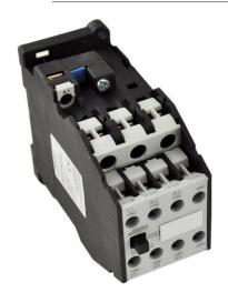
PART NUMBER – B3TF4322-0AK6: BRAH Electric, aftermarket direct replacement contactors for Siemens 3TF4322-0AK6, World Series, type 3TF, 3P, 3PH, 22A, 600V, 7.5HP @ 230V, 15HP @ 460V, 20HP @ 575V, complete with 110/120V AC coil, 2 N/O - 2 N/C auxiliary contact, AC magnetic contactor, suitable for use with 3TF series motor control systems
