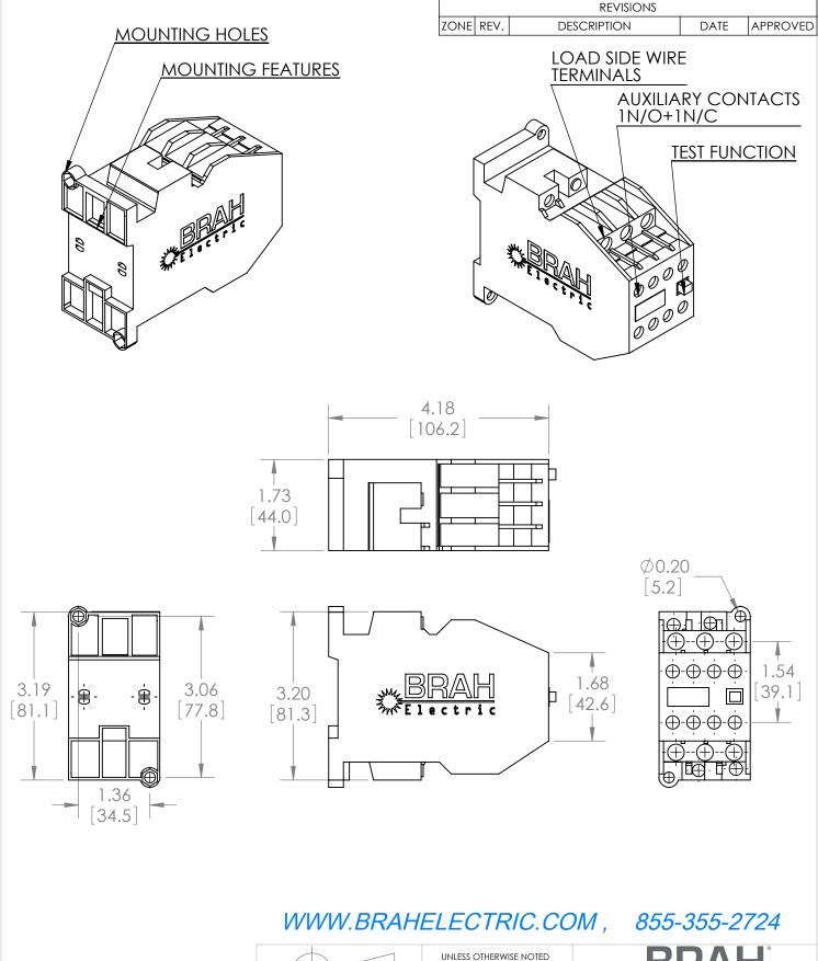
\*NOTE: BRAH ELECTRIC CONTACTOR B3TF4322-0AK6 IS AN AFTERMARKET DIRECT REPLACMENT FOR SIEMENS 3TF4322-0AK6,3TF SERIES. SUITABLE FOR USE WITH 3TB SERIES MOTOR CONTROL **SYSTEMS**
