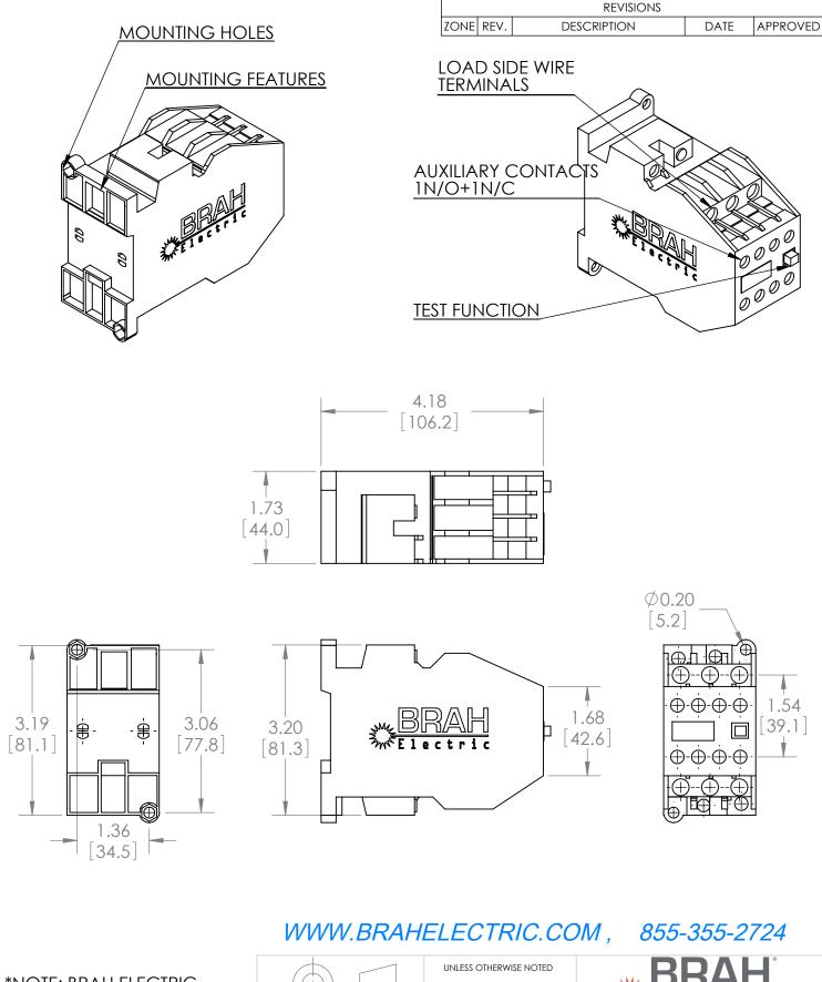
\*NOTE: BRAH ELECTRIC CONTACTOR B3TF4322-0AP6 IS AN AFTERMARKET DIRECT REPLACMENT FOR SIEMENS 3TF4322-0AP6,3TF SERIES. SUITABLE FOR USE WITH 3TB SERIES MOTOR CONTROL SYSTEMS
