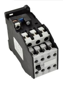
PART NUMBER – B3TF4322-0AP6: BRAH Electric, aftermarket direct replacement contactors for Siemens 3TF4322-0AP6, World Series, type 3TF, 3P, 3PH, 22A, 600V, 7.5HP @ 230V, 15HP @ 460V, 20HP @ 575V, complete with 240V AC coil, 2 N/O - 2 N/C auxiliary contact, AC magnetic contactor, suitable for use with 3TF series motor control systems
