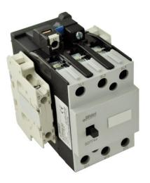
PART NUMBER – B3TF44: BRAH Electric, aftermarket direct replacement contactors for Siemens 3TF44, World Series, type 3TF, 3P, 3PH, 32A, 600V, 10HP @ 230V, 25HP @ 460V, 30HP @ 575V, complete with 110/120V AC coil, 2 N/O - 2 N/C auxiliary contact, AC magnetic contactor, suitable for use with 3TF series motor control systems
