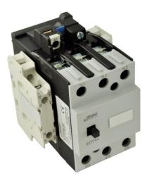
PART NUMBER – B3TF4422-0AVO: BRAH Electric, aftermarket direct replacement contactors for Siemens 3TF4422-0AVO, World Series, type 3TF, 3P, 3PH, 32A, 600V, 10HP @ 230V, 25HP @ 460V, 30HP @ 575V, complete with 480V AC coil, 2 N/O - 2 N/C auxiliary contact, AC magnetic contactor, suitable for use with 3TF series motor control systems
