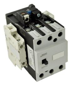
PART NUMBER – B3TF4522: BRAH Electric, aftermarket direct replacement contactors for Siemens 3TF4522, World Series, type 3TF, 3P, 3PH, 38A, 600V, 15HP @ 230V, 25HP @ 460V, 30HP @ 575V, complete with 110/120V AC coil, 2 N/O - 2 N/C auxiliary contact, AC magnetic contactor, suitable for use with 3TF series motor control systems
