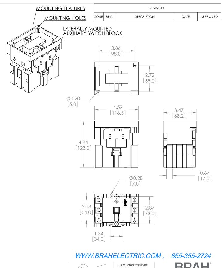
\*NOTE: BRAH ELECTRIC CONTACTOR B3TF46 IS AN AFTERMARKET DIRECT REPLACMENT FOR 3TF46, 3TF SERIES. SUITABLE FOR USE WITH 3TF SERIES MOTOR CONTROL SYSTEMS
