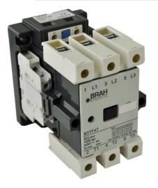
PART NUMBER – B3TF4622: BRAH Electric, aftermarket direct replacement contactors for Siemens 3TF4622, World Series, type 3TF, 3P, 3PH, 45A, 600V, 20HP @ 230V, 40HP @ 460V, 50HP @ 575V, complete with 110/120V AC coil, 2 N/O - 2 N/C auxiliary contact, AC magnetic contactor, suitable for use with 3TF series motor control systems
