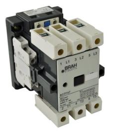
PART NUMBER – B3TF4622-0AC2: BRAH Electric, aftermarket direct replacement contactors for Siemens 3TF4622-0AC2, World Series, type 3TF, 3P, 3PH, 45A, 600V, 20HP @ 230V, 40HP @ 460V, 50HP @ 575V, complete with 24V AC coil, 2 N/O -2 N/C auxiliary contact, AC magnetic contactor, suitable for use with 3TF series motor control systems
