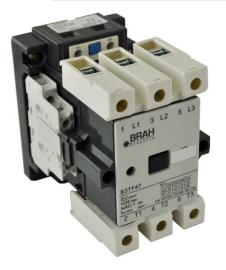
PART NUMBER – B3TF4622-0AK6: BRAH Electric, aftermarket direct replacement contactors for Siemens 3TF4622-0AK6, World Series, type 3TF, 3P, 3PH, 45A, 600V, 20HP @ 230V, 40HP @ 460V, 50HP @ 575V, complete with 110/120V AC coil, 2 N/O - 2 N/C auxiliary contact, AC magnetic contactor, suitable for use with 3TF series motor control systems
