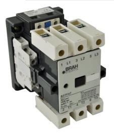
**PART NUMBER – B3TF47**: BRAH Electric, aftermarket direct replacement contactors for Siemens 3TF47, World Series, type 3TF, 3P, 3PH, 63A, 600V, 25HP @ 230V, 50HP @ 460V, 60HP @ 575V, complete with 110/120V AC coil, 2 N/O - 2 N/C auxiliary contact, AC magnetic contactor, suitable for use with 3TF series motor control systems.
