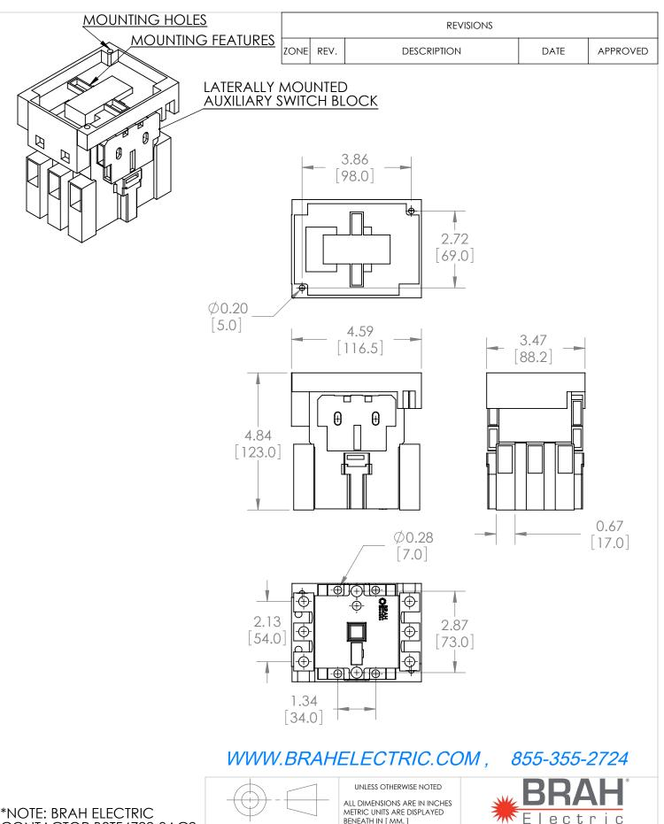
CONTACTOR B3TF4722-0AC2 IS AN AFTERMARKET DIRECT **REPLACMENT FOR 3TF4722-**0AC2,3TF SERIES. SUITABLE FOR USE WITH 3TF SERIES MOTOR CONTROL SYSTEMS
