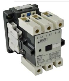
PART NUMBER – B3TF4722-0AK6:, BRAH Electric, aftermarket direct replacement contactors for Siemens 3TF4722-0AK6, World Series, type 3TF, 3P, 3PH, 63A, 600V, 25HP @ 230V, 50HP @ 460V, 60HP @ 575V, complete with 110/120V AC coil, 2 N/O - 2 N/C auxiliary contact, AC magnetic contactor, suitable for use with 3TF series motor control systems
