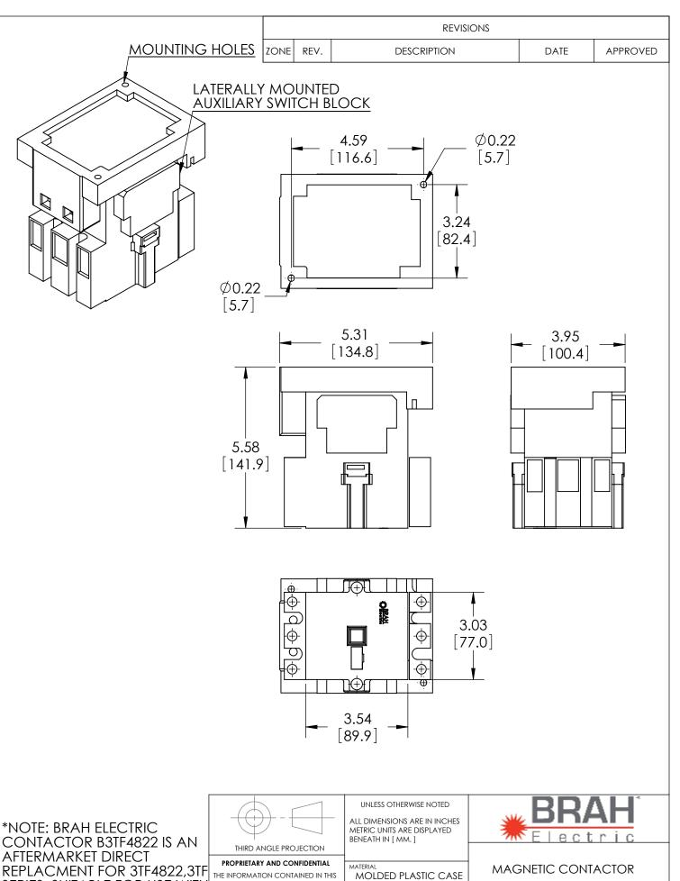
REPLACMENT FOR 3TF4822,3TF SERIES. SUITABLE FOR USE WITH 3TF SERIES MOTOR CONTROL **SYSTEMS**
