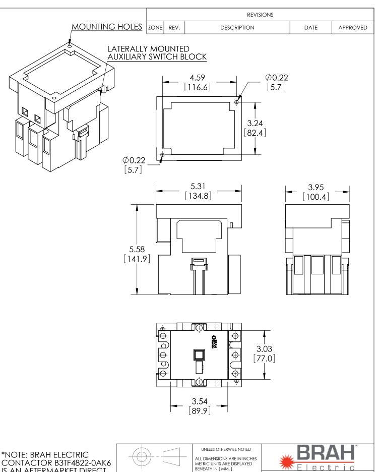
IS AN AFTERMARKET DIRECT REPLACMENT FOR 3TF4822-0AK6,3TF SERIES. SUITABLE FOR USE WITH 3TF SERIES MOTOR CONTROL **SYSTEMS**
