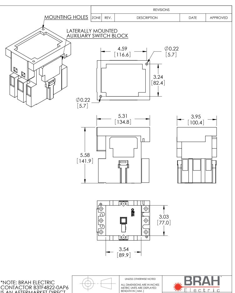
IS AN AFTERMARKET DIRECT REPLACMENT FOR 3TF4822-0AP6,3TF SERIES. SUITABLE FOR USE WITH 3TF SERIES MOTOR CONTROL **SYSTEMS**
