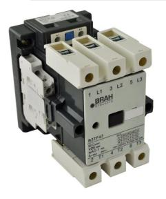
PART NUMBER – B3TF49: BRAH Electric, aftermarket direct replacement contactors for Siemens 3TF49, World Series, type 3TF, 3P, 3PH, 85A, 600V, 40HP @ 230V, 75HP @ 460V, 100HP @ 575V, complete with 110/120V AC coil, 2 N/O - 2 N/C auxiliary contact, AC magnetic contactor, suitable for use with 3TF series motor control systems
