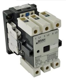
PART NUMBER – B3TF4922-0AC2: BRAH Electric, aftermarket direct replacement contactors for Siemens 3TF4922-0AC2, World Series, type 3TF, 3P, 3PH, 85A, 600V, 40HP @ 230V, 75HP @ 460V, 100HP @ 575V, complete with 24V AC coil, 2 N/O - 2 N/C auxiliary contact, AC magnetic contactor, suitable for use with 3TF series motor control systems
