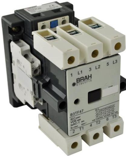
**PART NUMBER – B3TF4922-0AK6:** BRAH Electric, aftermarket direct replacement contactors for Siemens 3TF4922-0AK6, World Series, type 3TF, 3P, 3PH, 85A, 600V, 40HP @ 230V, 75HP @ 460V, 100HP @ 575V, complete with 110/120V AC coil, 2 N/O - 2 N/C auxiliary contact, AC magnetic contactor, suitable for use with 3TF series motor control systems
