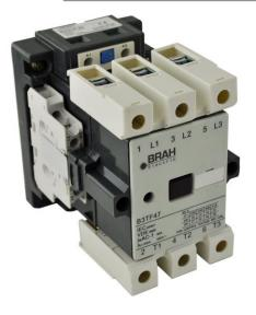
PART NUMBER – B3TF4922-0AVO: BRAH Electric, aftermarket direct replacement contactors for Siemens 3TF4922-0AVO, World Series, type 3TF, 3P, 3PH, 85A, 600V, 40HP @ 230V, 75HP @ 460V, 100HP @ 575V, complete with 480V AC coil, 2 N/O - 2 N/C auxiliary contact, AC magnetic contactor, suitable for use with 3TF series motor control systems
