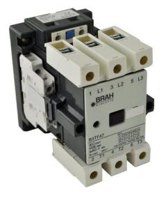
PART NUMBER – B3TF50: BRAH Electric, aftermarket direct replacement contactors for Siemens 3TF50, World Series, type 3TF, 3P, 3PH, 110A, 600V, 50HP @ 230V, 100HP @ 460V, 125HP @ 575V, complete with 110/120V AC coil, 2 N/O -2 N/C auxiliary contact, AC magnetic contactor, suitable for use with 3TF series motor control systems
