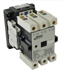
**PART NUMBER – B3TF5022-0AK6**: BRAH Electric, aftermarket direct replacement contactors for Siemens 3TF5022-0AK6, World Series, type 3TF, 3P, 3PH, 110A, 600V, 50HP @ 230V, 100HP @ 460V, 125HP @ 575V, complete with 110/120V AC coil, 2 N/O - 2 N/C auxiliary contact, AC magnetic contactor, suitable for use with 3TF series motor control systems
