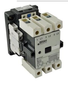
PART NUMBER – B3TF5122-0AVO: BRAH Electric, aftermarket direct replacement contactors for Siemens 3TF5122-0AVO, World Series, type 3TF, 3P, 3PH, 140A, 600V, 60HP @ 230V, 100HP @ 460V, 150HP @ 575V, complete with 480V AC coil, 2 N/O - 2 N/C auxiliary contact, AC magnetic contactor, suitable for use with 3TF series motor control systems
