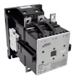
PART NUMBER – B3TF52: BRAH Electric, aftermarket direct replacement contactors for Siemens 3TF52, World Series, type 3TF, 3P, 3PH, 170A, 600V, 60HP @ 230V, 125HP @ 460V, 150HP @ 575V, complete with 110/120V AC coil, 2 N/O -2 N/C auxiliary contact, AC magnetic contactor, suitable for use with 3TF series motor control systems
