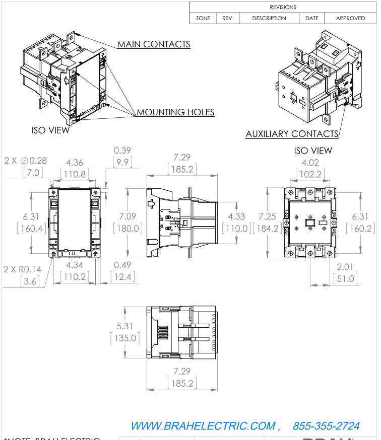
\*NOTE: BRAH ELECTRIC CONTACTOR B3TF5222-OAC2 IS AN AFTERMARKET DIRECT REPLACEMENT FOR SIEMENS 3TF5222-0AC2, WORLD SERIES. SUITABLE FOR USE WITH 3TF SERIES MOTOR CONTROL SYSTEM.
