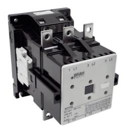
PART NUMBER – B3TF5222-0AP6: BRAH Electric, aftermarket direct replacement contactors for Siemens 3TF5222-0AP6, World Series, type 3TF, 3P, 3PH, 170A, 600V, 60HP @ 230V, 125HP @ 460V, 150HP @ 575V, complete with 240V AC coil, 2 N/O - 2 N/C auxiliary contact, AC magnetic contactor, suitable for use with 3TF series motor control systems
