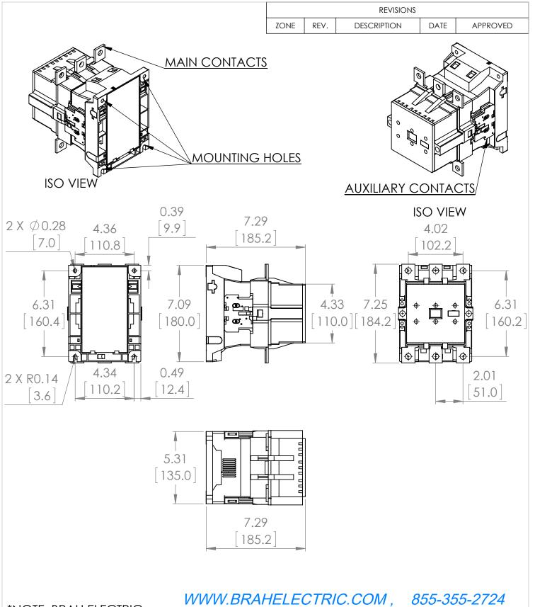
\*NOTE: BRAH ELECTRIC CONTACTOR B3TF5222-**OAVO IS AN AFTERMARKET** DIRECT REPLACEMENT FOR SIEMENS 3TF5222-0AV0, WORLD SERIES. SUITABLE FOR USE WITH 3TF SERIES MOTOR CONTROL SYSTEM.
