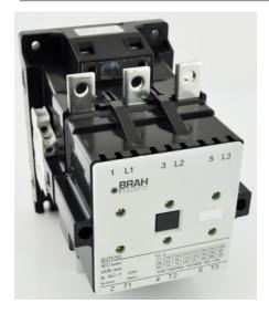
PART NUMBER – B3TF53: BRAH Electric, aftermarket direct replacement contactors for Siemens 3TF53, World Series, type 3TF, 3P, 3PH, 205A, 600V, 75HP @ 230V, 150HP @ 460V, 200HP @ 575V, complete with 110/120V AC coil, 2 N/O -2 N/C auxiliary contact, AC magnetic contactor, suitable for use with 3TF series motor control systems
