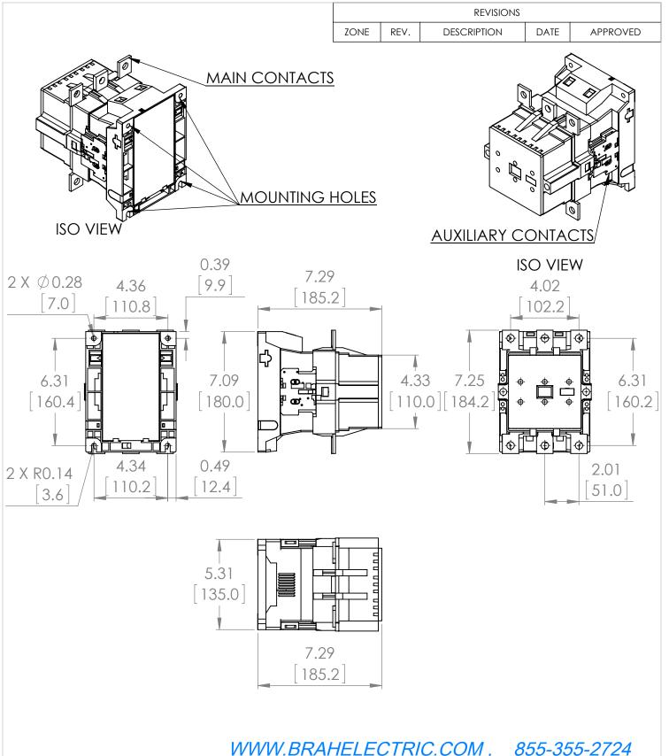
\*NOTE: BRAH ELECTRIC CONTACTOR B3TF5322-0AP6 IS AN AFTERMARKET DIRECT REPLACEMENT FOR 3TF5322-0AP6, TF SERIES. SUITABLE FOR USE WITH TF SERIES MOTOR CONTROL SYSTEM.
